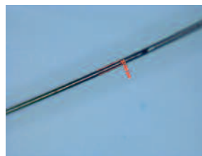
Figures 6 and 7. An etched wire that has been thinned to 20 \mu\text{m} along the length and a tip that has been thinned to approximately 1 micron.
