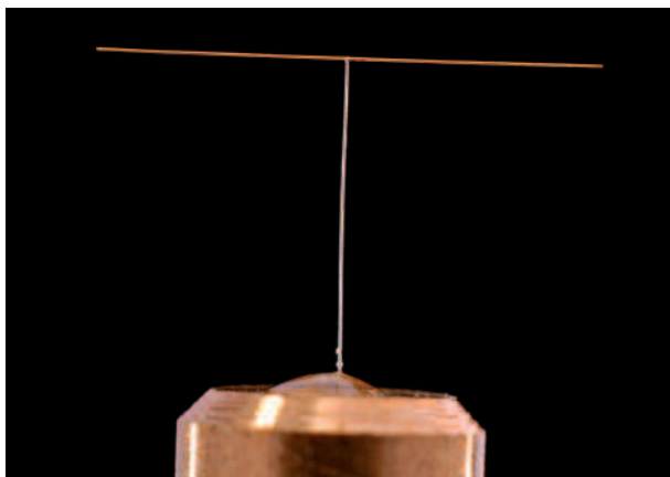
Figure 4. An example of a different type of thin-wire target assembled using standard techniques. (Horizontal wire 25 \mu\text{m} diameter.)
