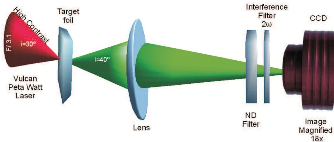
Figure 2. OTR diagnostic setup as used in the Vulcan experiment.
