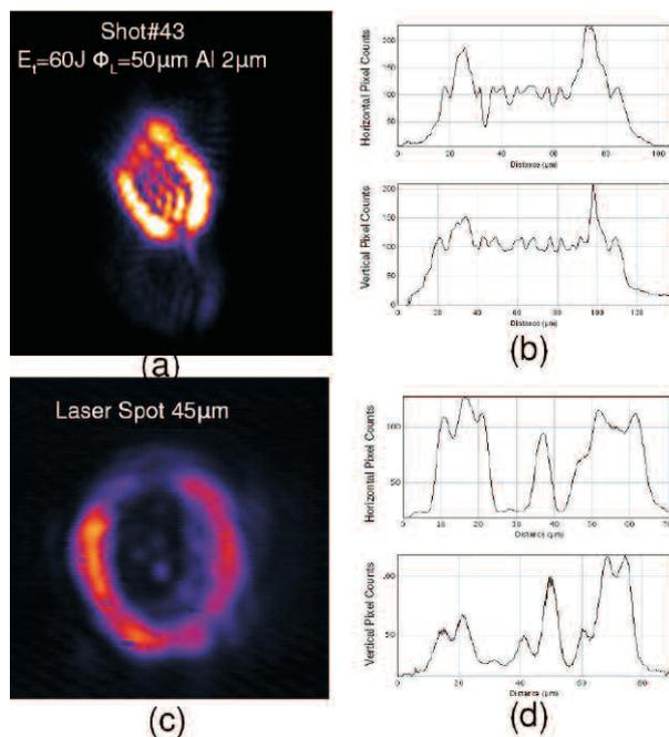
Figure 3. Comparison between CTR image (a) and laser spot spatial intensity distribution (b). The laser spot was imaged by an 8-bit Andor camera at normal incidence. Horizontal and vertical line-outs are shown alongside OTR image (c) and laser spot (d).
