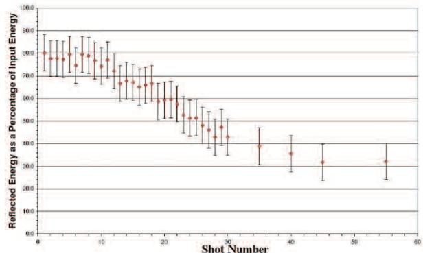
**Figure 4.** A graph showing how the reflected laser energy decreases as the coating becomes damaged.
