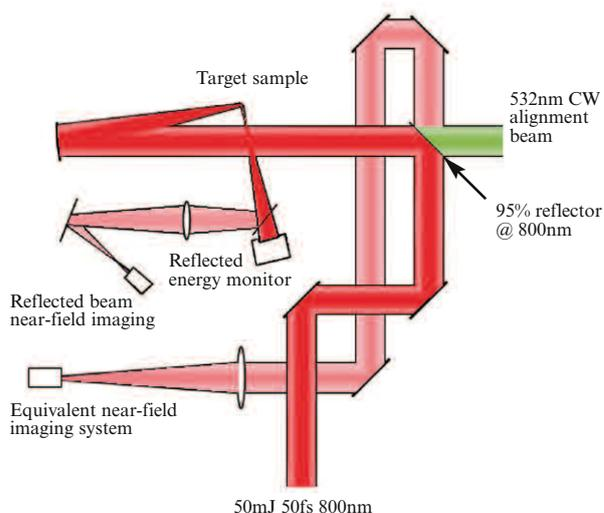
**Figure 1. Schematic representation of the experimental layout. Note that the target is positioned about 33 mm before focus in order to make an ellipse with minor and major axes of 5 mm and 7 mm respectively.**
