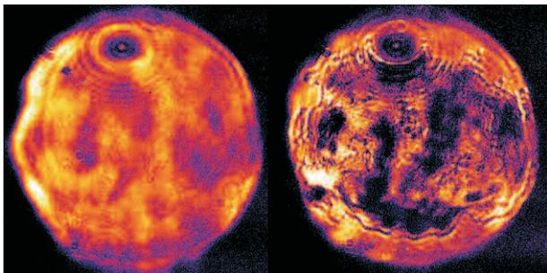
**Figure 2.** The reflected beam imaged at the target surface showing damage to the coating.
