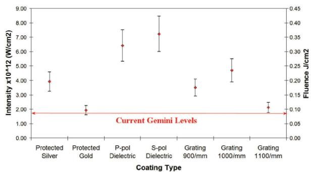
**Figure 3.** This graph shows the highest observed intensities and fluences at which the coatings did not damage. Also indicated is the levels at which Astra Gemini is currently operating.
