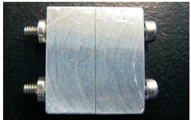
Figure 5. Aluminium block used to clamp iron wire.
