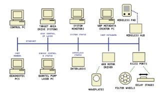
Figure 3. Gemini Control Network. The Ethernet has become a straightforward way to connect remote controllers and hardware to the control PC.
