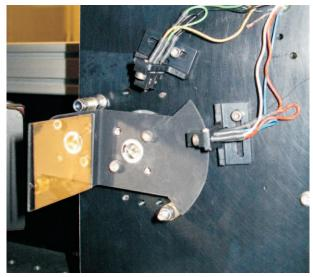
Figure 1. Low inertia blade with gold reflector capable of selecting a single 10 Hz pulse.
