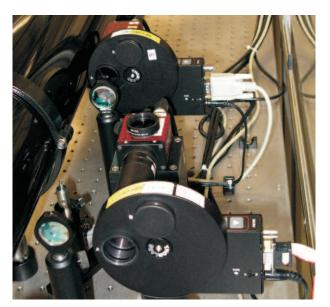
Figure 2. Filter wheels installed to automatically attenuate pulse on high power shots.
