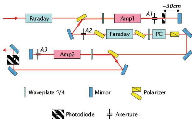
Figure 1. The 9 mm preamplifier layout.
