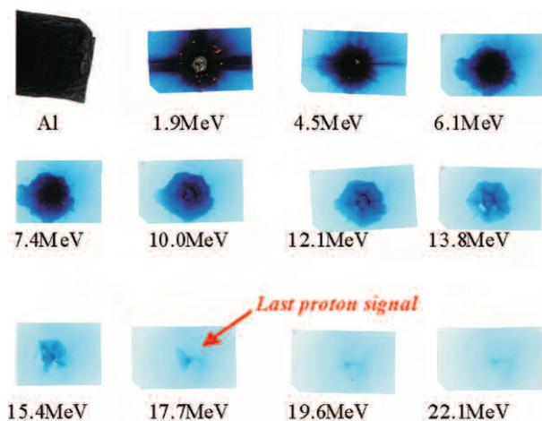
Figure 4. Proton beam with the old setup.
