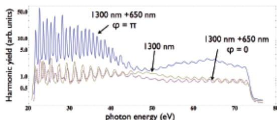
**Figure 2. High harmonics generated with fundamental and with the two-colour ( $\omega + 2\omega$ ) laser field for two values of the relative phase between the two fields. The first peak is the 23th harmonic of the 1300 nm.**
