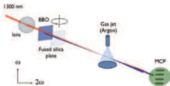
**Figure 1. Experimental setup for the two-colours experiment in Artemis.**
