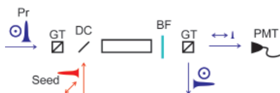
Figure 2. Schematic diagram of molecular alignment setup. Pr: probe; GT: Glan-Thompson polarizer; DC: Dichroic mirror; BF: Schott glass filter (BG37); PMT: Photomultiplier tube detector.
