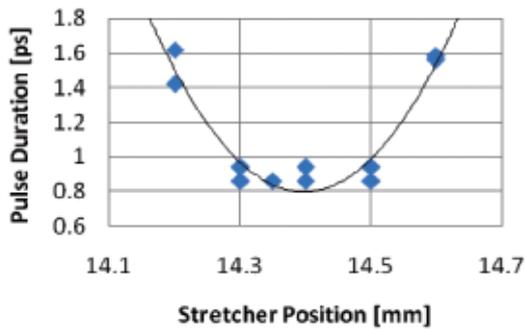
Figure 4. Stretcher tuning for beam 7.
