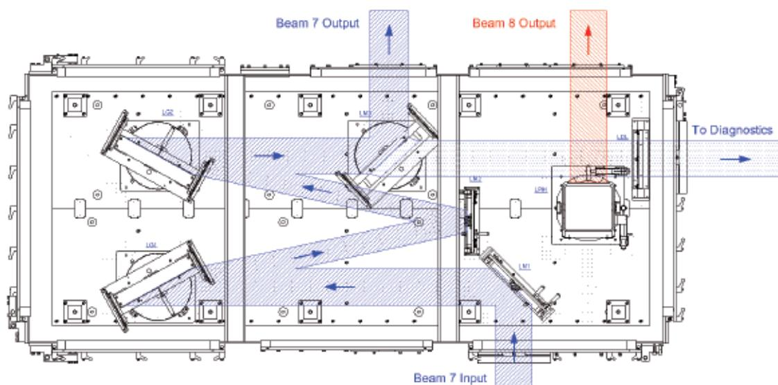
Figure 3. Single pass compressor. Lower layer.
