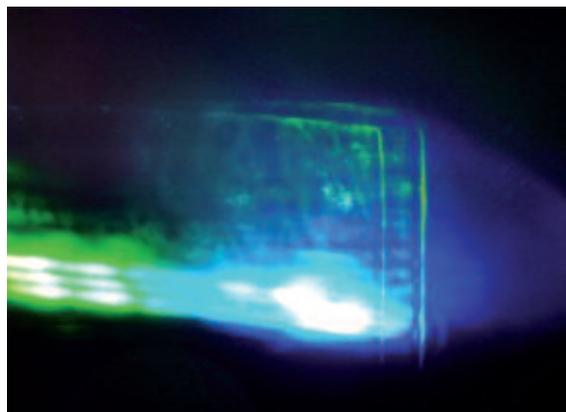
Figure 5. Damages on the first grating of the double pass compressor.
