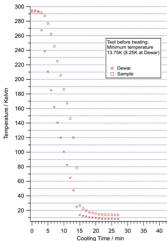
**Figure 7. Measurement of the temperature of the sample in the MatSci chamber showing that it gets below 14 K in 30 minutes**
