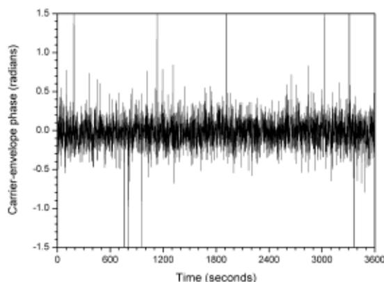
**Figure 2.** Measurement of the CEP of the laser system at 13.5 mJ showing an rms value of 310 mrad over a full hour.
