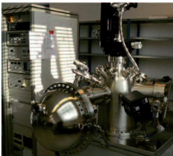
**Figure 6. The Materials Science Station, showing the hemispherical electron analyser.**
