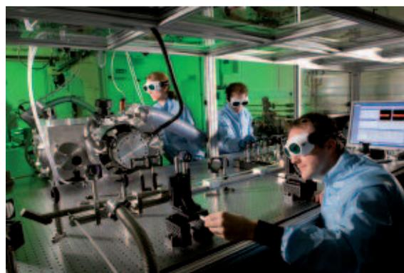
**Figure 1.** View of the Artemis facility showing the laser beamlines and the XUV generation chamber.
