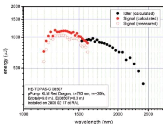
Figure 3 (a). Calibrated output of the OPA system
