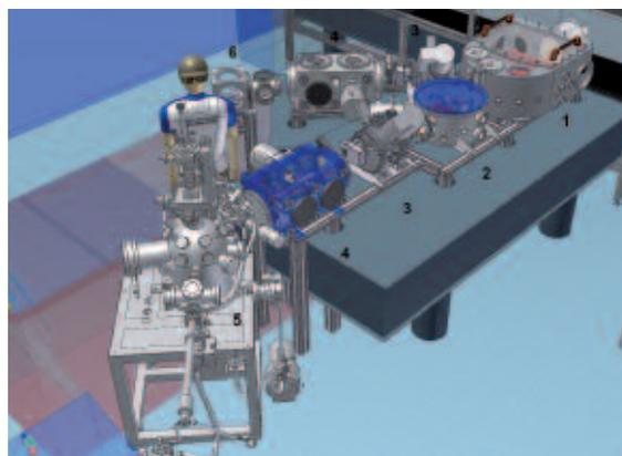
Figure 5. Engineering drawing of the XUV beamlines. Chamber #1 is the XUV generation chamber, #2 is the monochromator, #3 is the flat-field spectrometer (shown in both of its possible locations), #4 are toroidal mirror chambers, #5 is the materials science station and #6 shows the location of the AMO station.
