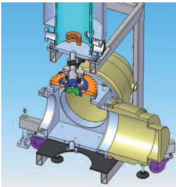
**Figure 8.** Engineering drawing showing a cross-section of the AMO station with the molecular beam chamber located underneath the velocity-map imaging detector.
