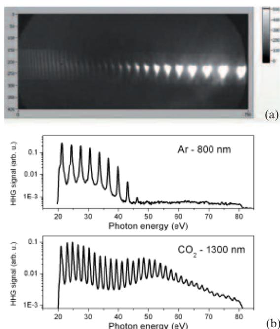
Figure 4 (a). HHG spectrum detected with the flat-field spectrometer using a 1300 nm drive laser pulse and (b) calibrated spectra showing that harmonics up to at least 80 eV can be produced.
