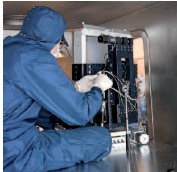
Figure 3. 5 DOF grating mount inside compression chamber.
