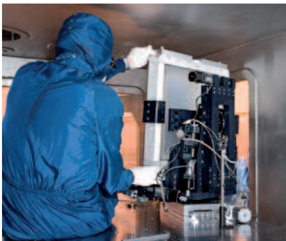
Figure 4. Installation of grating mount.
