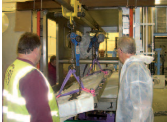
Figure 12. Quinto install compression chamber breadboards, progress is hampered by the stiffening tubes.
