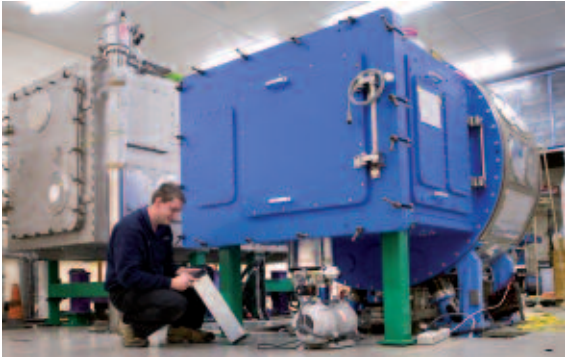
Figure 10. Early vacuum testing carried out to check the O ring between interaction chamber and extension chamber.
