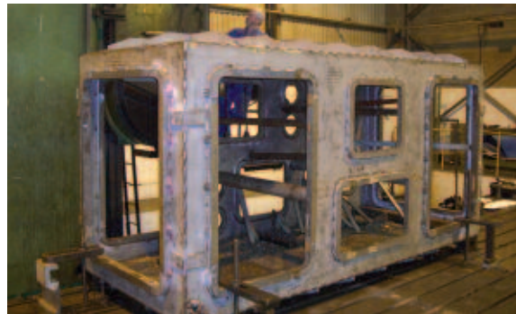
Figure 1. The new compression chamber undergoing final machining.
