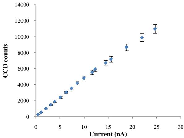
**Figure 5.** BC-408 scintillator response as a function of beam current.
