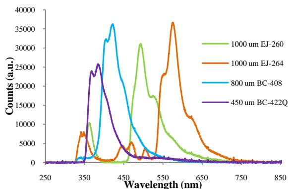
**Figure 2.** Optical emission spectra for BC-422Q, BC-408, EJ-260 and EJ-264 thin organic scintillators. Spectra were obtained by illuminating each scintillator with a 2.5 MeV proton beam.
