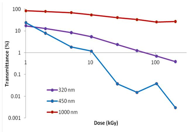
**Figure 4: Transmittance against dose for RCF in three regions of the spectrum.**
