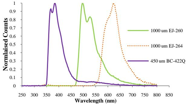
**Figure 3.** Predicted optical emission spectra for a combination of BC-422Q, EJ-260 and EJ-264 organic scintillators. Emission curves have been normalised as they do not take into account the incident ion flux on each layer.
