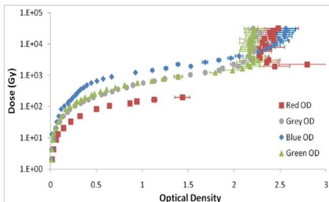
**Figure 3: Nikon Super Cool Scan 9000 ED calibration of HD810 optical density with dose.**
