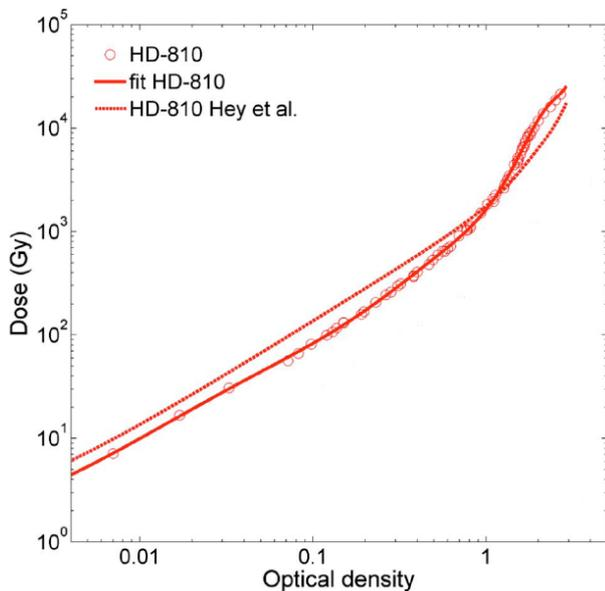
**Figure 2: Greyscale calibration curve comparing [6,7].**
