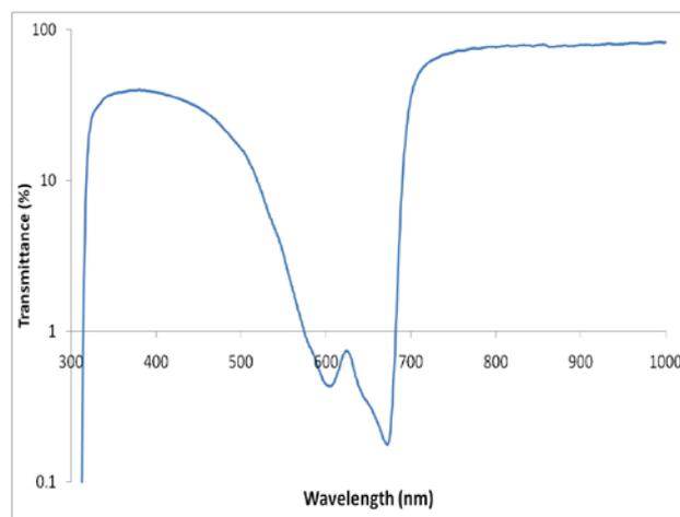
Figure 1: RCF HD810 transmission spectrum on exposure to 570 Gy.
