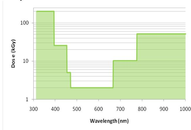
**Figure 5: The shaded area gives a guide of the maximum detectable dose in each region of the spectrum.**
