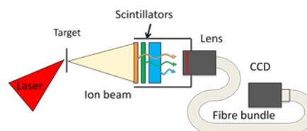
**Figure 1.** Schematic of the ion beam spatial profile monitor. Higher energy protons are stopped in the shorter wavelength scintillators further in the stack. The combined optical signal is collected and relayed to a CCD camera via a fiber optic bundle.
