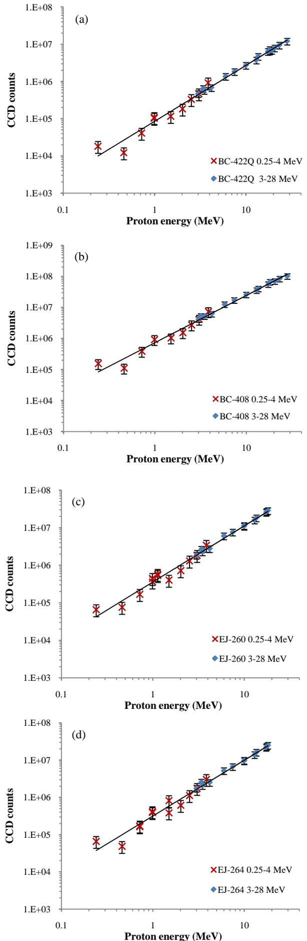
**Figure 4.** Proton response data for (a) BC-422Q, (b) BC-408, (c) EJ-260 and (d) EJ-264 thin organic scintillators together with empirical fits.
