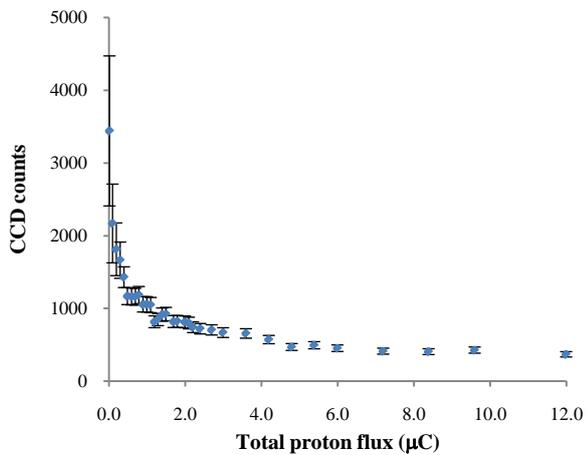
**Figure 6.** EJ-260 scintillator response as a function of total incident proton flux when irradiated with a focused current of 10 nA for 12 minutes.
