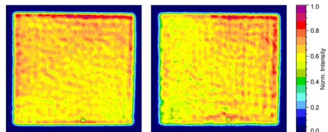
Figure 3 Images of the output near fields at 1 Hz (1.0 ms pump) with an output energy of 9.4 J and also 10 Hz (0.8 ms pump) at an energy of 7.4 J.
