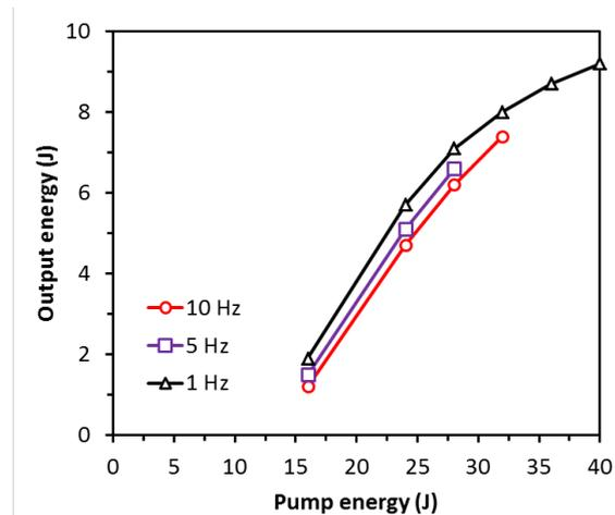
Figure 2 Dependence of 1030 nm output pulse energy on 940 nm pump energy for varying pulse repetition rates at 125K.
