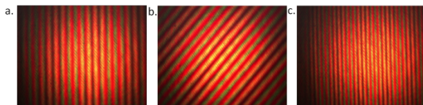
Figure 4. Interference patterns of the three colour interferometer; a. when the interferometer is perfectly aligned, b. with a vertical tilt on the target mirror showing a rotation of the fringes and c. with a horizontal twist on the target mirror, narrowing the spaces between the fringes.
