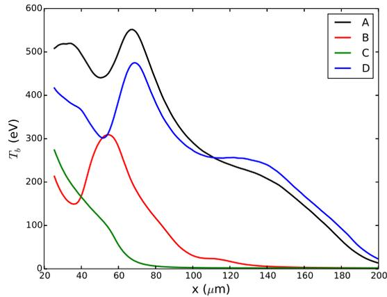
**Figure 4.** Lineouts (along guide axis) of background electron temperature (eV) in simulations with different wire targets with/without inverse conical tapers.
