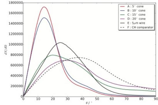
**Figure 3.** Angular distribution of fast electrons from different simulations in [1]. Legend indicates type of guide element used in each simulation. Distributions are calculated at  $3$  ps (substantially after end of injection).
