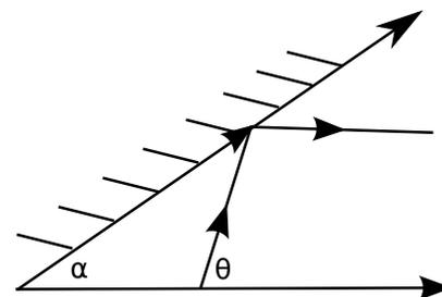
Figure 2. Schematic plot of reflection from oblique plane.
