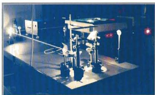
Loan Pool lasers probe ultra-low temperature reactions in the CRESU apparatus at the Université de Rennes, France. (93 FC 1124).
