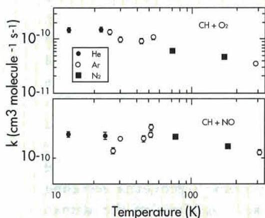
Rate constants for the reactions CH + O<sub>2</sub> and CH + NO as a function of temperature measured in the CRESU apparatus.
