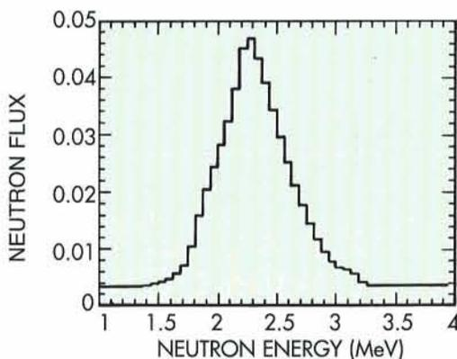
Spectra of neutron energies emitted from the deuterated plastic target in the forward (top) and backward (bottom) directions
