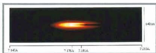
Computer code simulation of spatially resolved, Doppler shifted emission at the aluminium Lyman-alpha wavelength. A 50  $\mu\text{m}$  wire is assumed irradiated at  $4 \times 10^{14}$   $\text{W cm}^{-2}$  in a 600 ps pulse.
