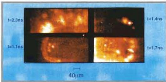
One of the major problems in inertial confinement fusion results from the non-uniformities in the laser beams used to irradiate the fusion capsule. These non-uniformities are imprinted onto the ablation surface seeding the growth of Rayleigh-Taylor instability which impairs the symmetry of the implosion.
