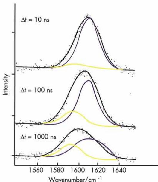
**Time-resolved resonance Raman spectroscopy performed at different temperatures has allowed the first observation of the birth of the solvated ion from the geminate ion pair.**
