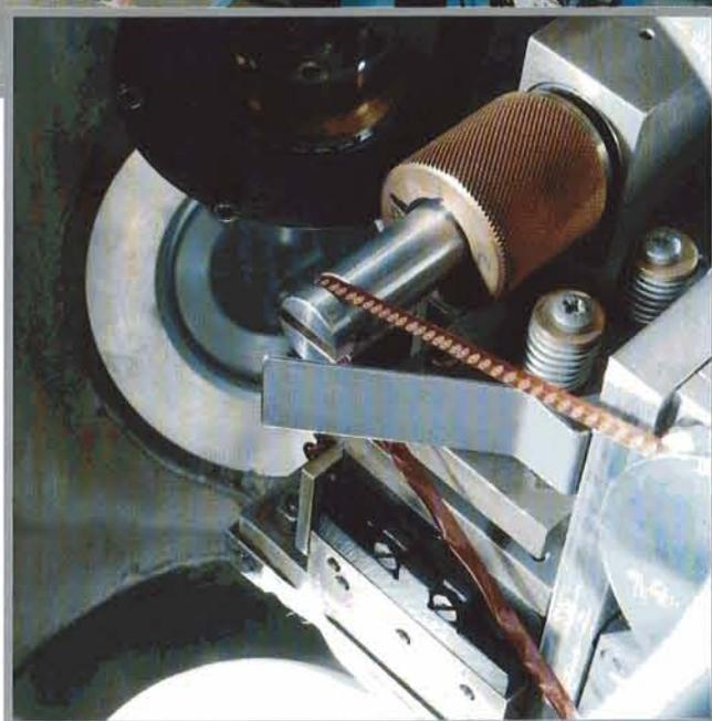
Tape transport system of the laser produced X-ray source. The copper tape, which provides a fresh target for each laser pulse, produces characteristic X-rays of around 1 nm wavelength. (91 RC 1004).
