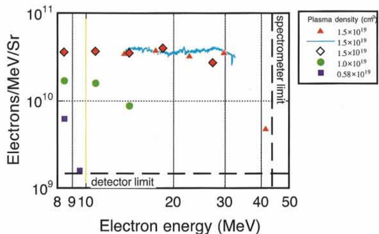
Spectrum of accelerated electrons at different plasma densities.
