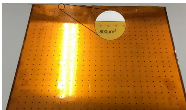
Figure 6: 260 \times 260\ \text{mm} polyimide sheet with 625 laser machined 800 \times 800\ \mu\text{m} windows down to a thickness of 5\ \mu\text{m}
