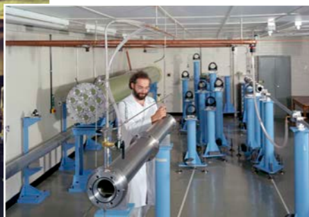
Chris Hooker adjusting the Raman amplifier in the Sprite multiplexing room. The green pipe behind Chris transports the laser beams into and out of the Sprite laser cell on the other side of the wall, 1988. (88FC3341)
