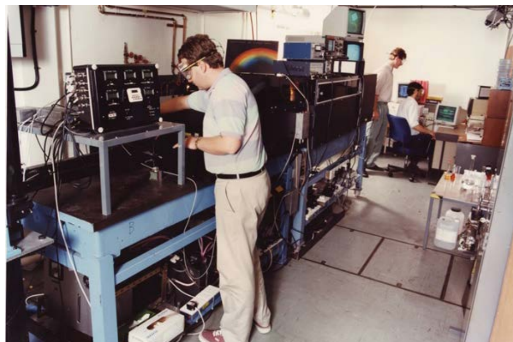
Tony Parker setting up a copper-vapour laser in the Time-Resolved Resonance Raman ( TR^3 ) facility, 1992. (92RC3455)
