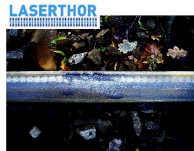
Based on an idea by Malcolm Higgins, a novel use of lasers was pioneered by Tony Parker and colleagues in 2000 in an attempt to solve Railtrack's leaves-on-the-line problem. A laser was used to ablate (burn-off) leaves from a 20mm strip on each rail. A company – LaserThor – was set up, and trials started in 2000. Work is continuing in the Netherlands.
