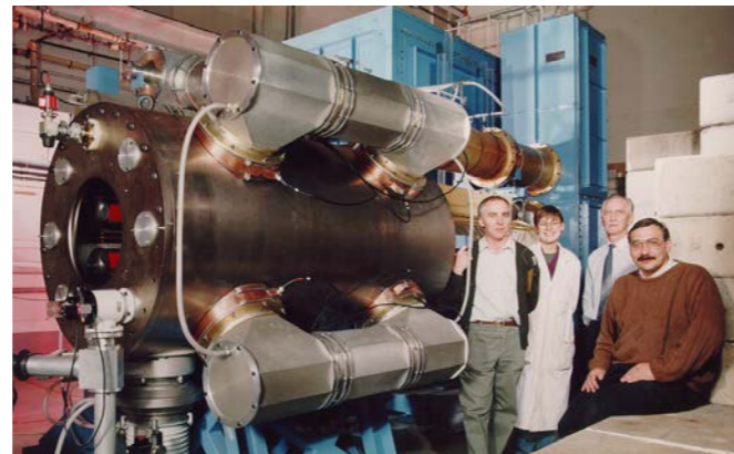
Titania module under assembly in R7. In the photograph are (from left to right) John Govans, Sally-Ann Brind, Dave Wood and Andy Frackiewicz. The red velvet of the electron emitters is just visible.
