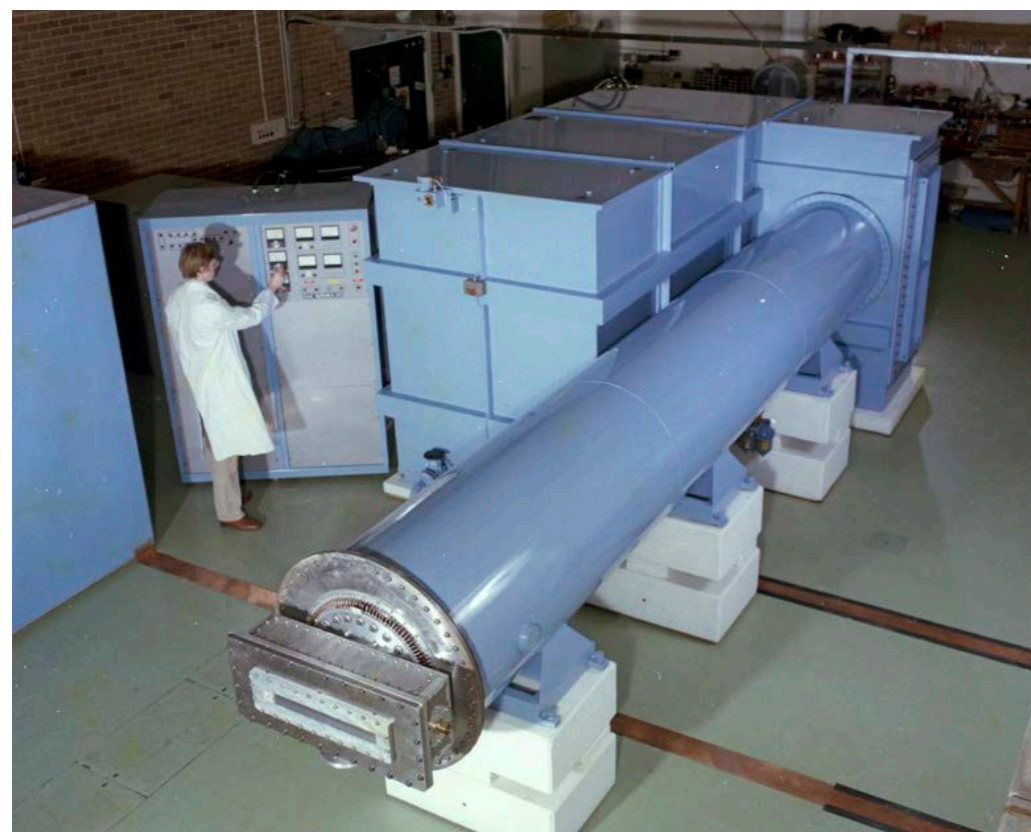
Chris Edwards monitoring ELF. The long blue cylinder is the Blumlein pulse-forming line (named after its inventor, the British engineer Alan Blumlein). The blue cabinet at the far end is the Marx bank generator; the silver rectangular box fastened to the end of the Blumlein is the diode chamber. The single electron beam came out through the slit window. (28255)
