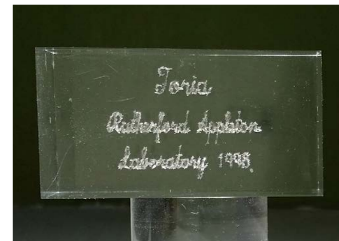
Ultrafast Laboratory facilities were used during the RAL Open Days in 1998 to "print" visitor's names in the middle of blocks of Perspex using a femtosecond laser linked to a Hewlett-Packard plotter. These little souvenirs were very popular, and demonstrated the precision of the laser beam.
