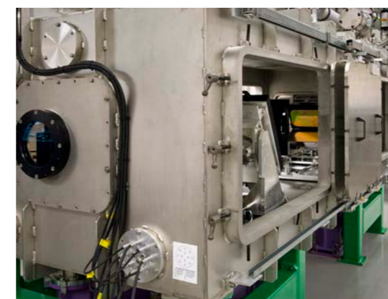
South compressor chamber installed, 2007. One of the gold-coated gratings used for pulse compression can be seen at the far end of the chamber. (07EC3604)
