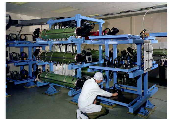
A picture of the "main 6" 108mm diameter amplifiers in the Vulcan Laser Area, 1983. (83FC1737)
