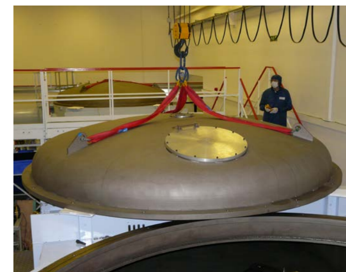
Each day, the two 4.5 metric tonne compressor lids were craned off before work could start. This operation alone took an hour each time, but the delay was mostly due to housework as you cannot open up a clean vacuum vessel unless you are confident that the area outside is as dust-free as possible.
