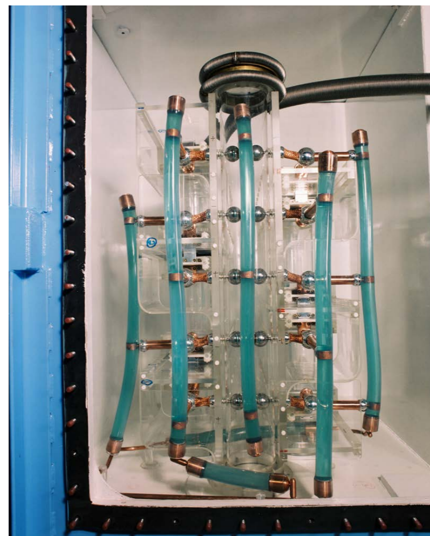
A studio portrait of a Marx spark-gap column; in reality this was about 1.5m in height. The pairs of stainless steel electrodes are the switches that connect the Marx capacitors when the machine is fired. (27554)
