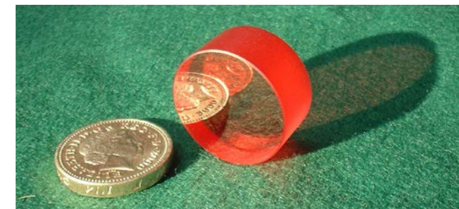
Titanium-doped sapphire (TiS) crystal, the heart of Astra's third amplifier.
