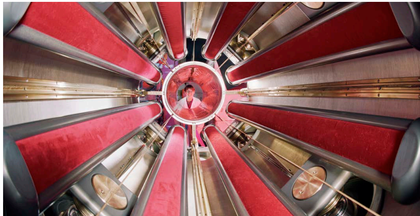
Sally-Ann Brind looking down the barrel of the vacuum vessel. The red panels are the cathodes of the electron guns, and are made of actual velvet, which acts as a good electron emitter because its fine hairs enhance the electric field, 1994. (94RC2911)
