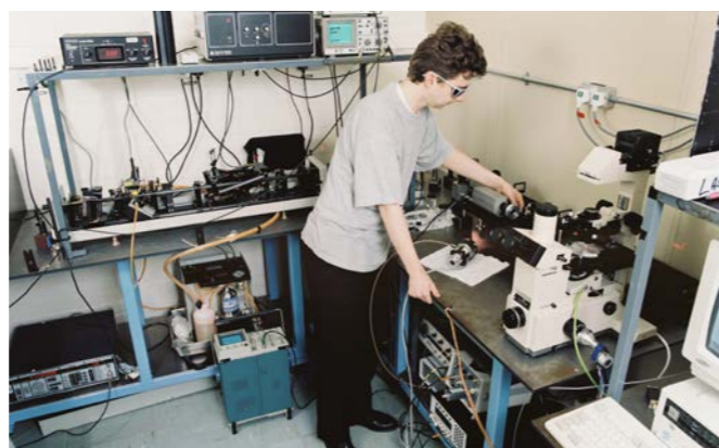
Kevin Henbest in the Laser Microscopy Laboratory, c.1997. A Gated Image Intensifier (GOI) camera can be seen on the bench to the left of the white confocal microscope; in the background is the "cavity dumper" laser.
