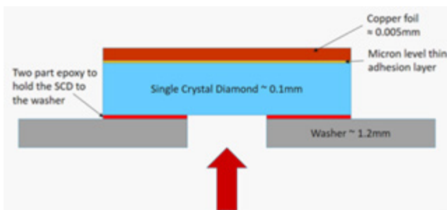
Figure 1: Schematic of the assembled multilayer target
