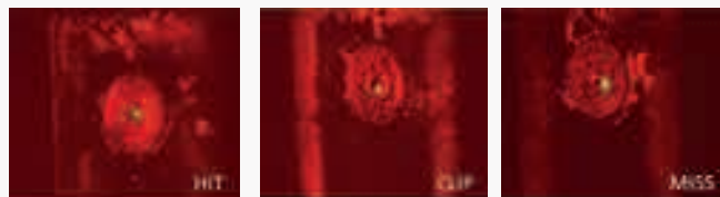
Fig 2: a) image of self-emission directly on cone tip, b) clipping the cone tip, and c) completely displaced from the cone tip.
