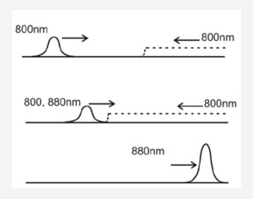
Schematic of the backwards Raman amplifier scheme, with seeding from forward scatter of a short pulse in an under-dense plasma.
