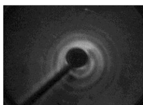
Figure 4: Diffraction pattern obtained from a 20 nm thick polycrystalline Pt sample.
