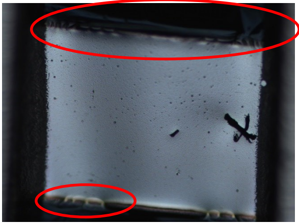
Figure 7. Bright field image of aluminium strip produced using a plastic layer removed by oxygen plasma etching. There is some plastic visible at the top and bottom circled in red
