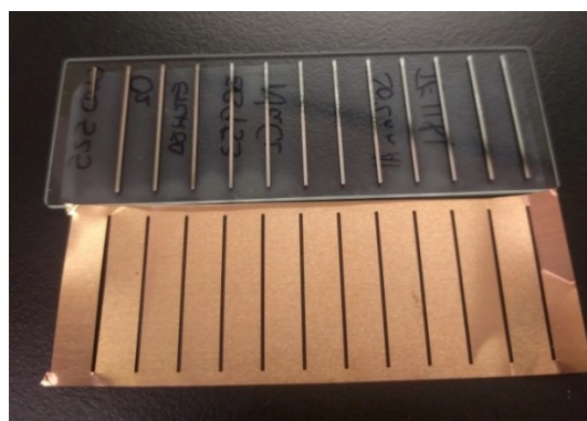
Figure 2. Microscope slide with aluminum strips defined by a copper mask. The coating was performed with the mask overlaid on the slide to define the strips
