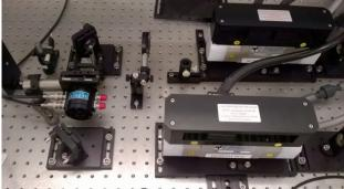
Figure 3. Pulse shaping Pockels cell
