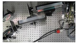
Figure 2. Layout of the new polarisers for TA2. The beam enters through the waveplate at upper right and is steered via the polarisers to the folding mirrors at left, where it is injected into the original beam path.
