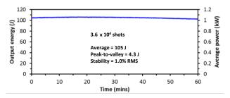
Figure 3: Long term energy stability over 1 hour at 10 Hz.
