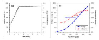
**Figure 12:** (a) Output energy ramp to 105 J and (b) energy and conversion efficiency when final cryo-amplifier operated to 1 kW average power level at 10 Hz at HiLASE.
