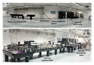
**Figure 5**: Photographs of the HiLASE laboratory (a) before and (b) after optical table assembly.
