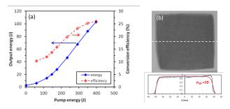
**Figure 11:** (a) Output energy and conversion efficiency, and (b) burn pattern captured at 103 J with cross-section when final cryo-amplifier operated at 1 Hz at HiLASE.
