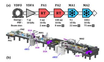
Figure 1: a) Schematic of DiPOLE100 amplifier chain showing typical output performance after each amplifier stage, including free-space beam size and shape: YDFO = Yb-silica fibre oscillator; YDFA = Yb-silica fibre amplifier (inc. temporal pulse shaping); PA = room-temperature pre-amplifier ( $1=Yb:CaF_2$  regenerative, 2=Yb:YAG multi-pass); MA = main cryogenic amplifier (ceramic Yb:YAG multi-slab). (b) 3D model of DiPOLE100 system: D = Diode pumps; cGC = cryogenic gas coolers.
