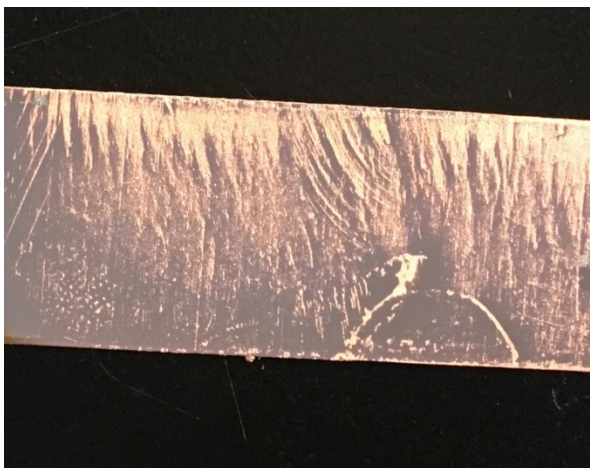
Figure 2: Copper plating with seed layer, 10mA applied.
