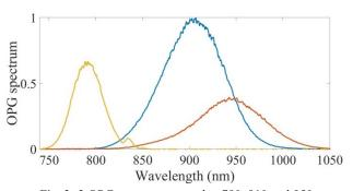
Fig. 3- 3 OPG spectra, centered at 790, 910 and 950nm obtained by changing the phase matching angle.
