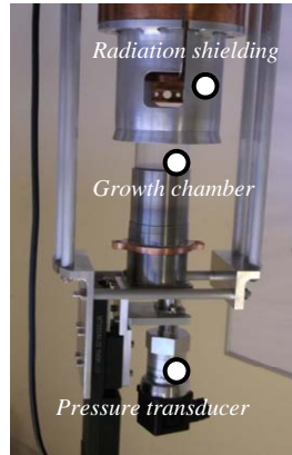
Figure 4. Lower section of the cold assembly with the growth chamber in place.
