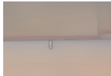
Figure 12. Edge of the CH membrane with a 3µm x 3µm x 10µm target at the edge and ready for use.
