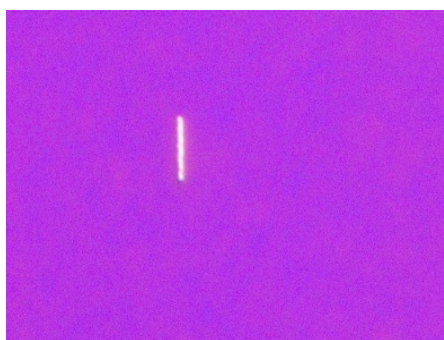
Figure 9. Optical image of filled 1µm x 1µm x 10µm trench.
