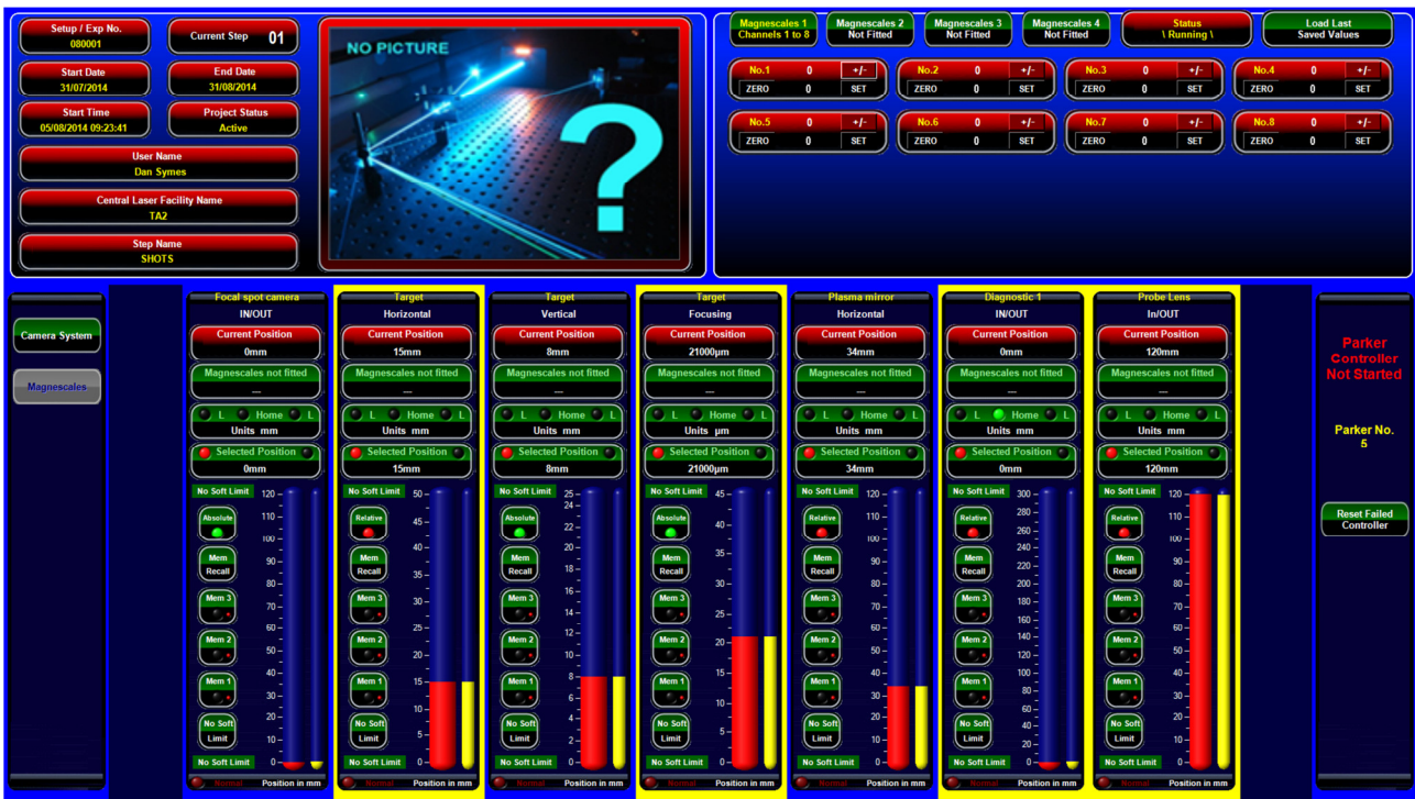
Figure 4. Screenshot of the drive system software where all motions necessary between shots have been assembled on a single interface allowing “single-click” operation of each.
