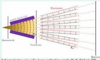
Schematic top view of a large collection angle Multi-Pinhole TPS, capable of providing an angularly resolved, complete spectral characterization of high-energy, multi-species ion beams.
