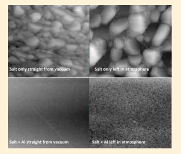
Figure showing the AFM scans of the salt and salt + aluminium coatings straight from vacuum and after being left in the atmosphere.
