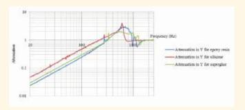
Attenuation of vibrations in the far field across a range of frequencies from 10 Hz up to 2500 Hz. Different adhesives for attaching the mirror substrate to the piezo platform produce varying responses.
