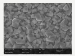
SEM image of copper surface formed on aluminium strip. Plating conditions:  $18^{\circ}$ C, 1mol dm<sup>-3</sup> CuSO<sub>4</sub>, not stirred throughout plating time, 10mA applied.
