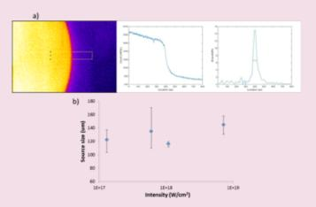
a) an example image cast by the penumbral aperture, with the two subsequent inlet graphs being a lineout and the gradient showing the source size b) shows the results from the defocus scan on 100µm tantalum, error bars shown account for the asymmetry of the source and variance in the source further corrections can be made by accounting for the point spread function (PSF) of the filter layers.
