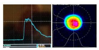
*Temporal (left) and spatial characteristics of a 50J pulse on the Gemini long-pulse beamline.*
