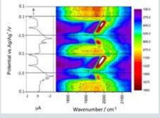
VSFG spectra showing how surface electrochemical events seen by the current-voltage response (left) can be monitored using VSFG spectroscopy (right) where we see new v(CO) bands forming at the potentials of the electrochemical events.
