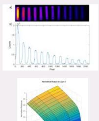
Figure 1 (top): a) Example data from the scintillator based x- ray spectrometer. The x-rays are entering from the left and being absorbed as they pass through the array. The photons that are emitted are recorded on a camera. b) shows a lineout of the image. The signal clearly falls as a function of layer.
