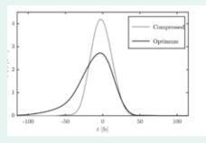
Figure 2: Temporal shape of the laser pulse that produced the highest x-ray yield
