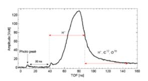
TOF signal acquired with a 100  $\mu$ m thick diamond detector placed @ 2.35 m downstream from the target.
