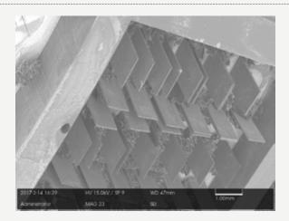
1.3mm thick PMMA after exposure and development
