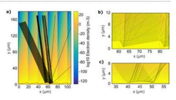
[a] Ray trace of a sawtooth plasma grating structure, demonstrating that the majority of the incident rays are reflected from the grating at a consistent angle, which is different to the incident angle. The red line shows the critical surface of the plasma.
