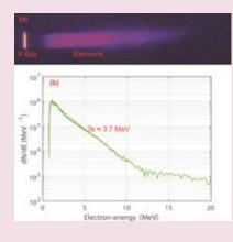
An electron spectrometer has been employed in measuring escaping electrons from laser-solid interactions. Electron spectra have been obtained in different laser pulse conditions. Dependence of escaping electron numbers and temperature on the pulse energy, intensity and duration is shown in this report.
