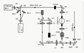
Figure 1 Schematic of the experimental setup to increase the fluence on LBO Crystal. M1-M7: Mirrors; L1-L5: Lenses; HWP: Half-wave Plate; QWP: Quarter-wave plate; VSF1: Vacuum spatial filter; W1, W2: Wedges; Cam 1, Cam 2: Cameras, EM1, EM2: Energy meters; BD1, BD2: Beam dumps.
