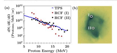
(a) Proton spectra from a RadioChromic Film stack and a Thomson Parabola Spectrometer (solid line) for 10 nmthick carbon targets irradiated under similar conditions on the Gemini laser.
