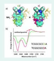
a) Portion of crystal structures of  $\Lambda$ -[Ru(TAP)<sub>2</sub>(dppz)]<sup>2+</sup> intercalated at GC and IC steps (b) TRIR spectra of  $\Lambda$ -[Ru(TAP)<sub>2</sub>(dppz)]<sup>2+</sup> bound to G9- and I9substituted DNA sequences at 1150 ps after excitation (Keane et al., Chem. - Eur. J., 2017, 23, 10344)
