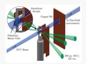
Experiment setup. Two palladium-coated CH foils surround a thin submicron aluminium sample (1 mm away). Three 527 nm laser pulses provide a total of  $\approx 2 \times 10^{15}$  W/cm<sup>2</sup> laser intensity onto each palladium foil (100 J in 200 ps full width at half maximum), which is converted into hard x-rays that bathe the sample, raising its temperature. An XUV probe propagates through the heated sample and onward to a spectrometer for analysis.
