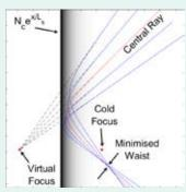
Schematic of a focusing beam incidence into an exponentially decaying plasma profile from a planar plasma mirror
