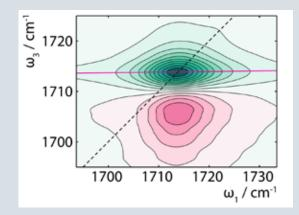
Isotropic 2DIR spectrum for the C–N anti-symmetric stretch vibration of the formamidinium cation in lead iodide perovskite films
