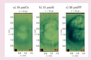
3.5 MeV proton flux distributions in the form of scanned radiochromic film for different target materials a) 10  $\mu$ m Cu b) 15  $\mu$ m Al c) 30  $\mu$ m PP (Plastic). The point in time at which the proton probe crosses the main interaction is given above the images. In all cases the focal spot separation was set to 435  $\mu$ m and a Cu mesh was included in the proton probing beam before the interaction. This is only visible in c) due to increased scattering in the metal targets.
