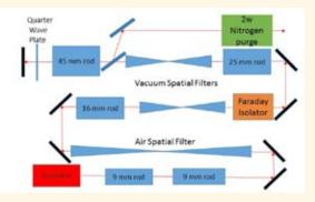
Schematic representation of the Component Test Lab with frequency doubling stage.
