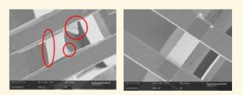
Left: SEM Image of aluminium strip produced by removal of a plastic support layer. Areas of contaminant can be seen circled in red.
