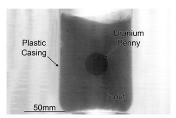
Radiograph of uranium penny encased in grout obtained using single pulse of a laser-driven x-ray beam.
