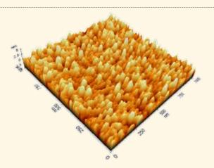
1 μm x 1 μm atomic force microscope 3D reconstruction of a GCIB nano-textured Yb:YAG sample surface.
