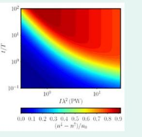
Degree of electron spin polarization, as a function of laser intensity and time normalized to the laser period.
