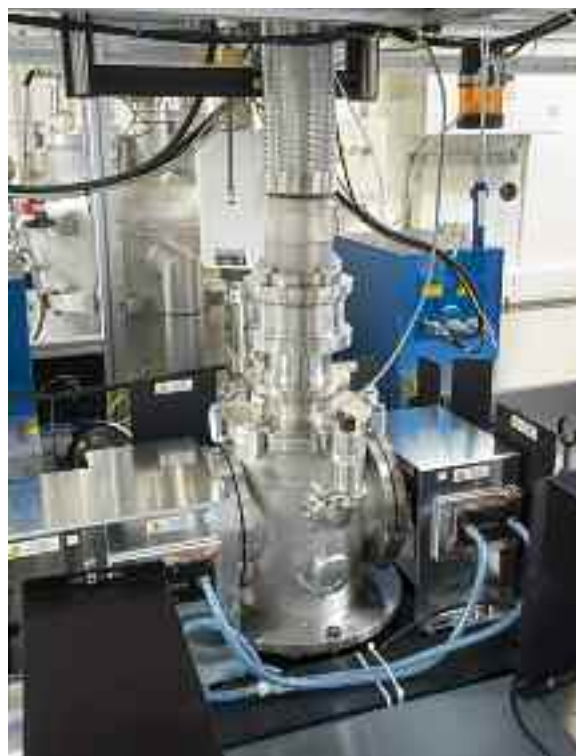
Figure 1: The DiPOLE amplifier head (14EC1568)
