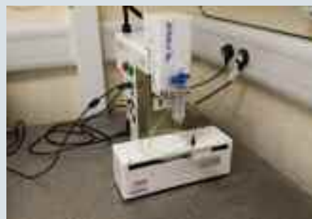
Dispensing robot with 3 axis stage.
