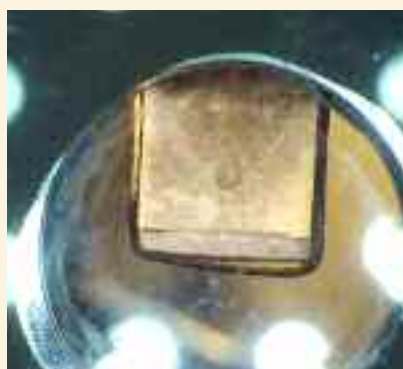
Image of solidified hydrogen over copper target foil.
