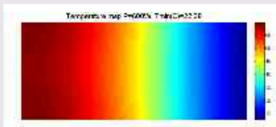
Temperature distribution map along 25mm (vertical) length and 45mm (horizontal) radius of the Ti:Sapphire crystal. The map corresponds to 600W of input pump power.
