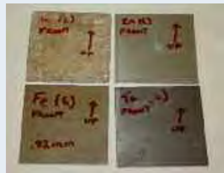
Four of the foils activated by neutrons during the investigation.
