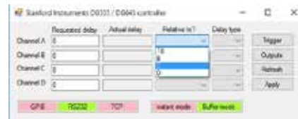
Figure 2: Graphical User Interface of the Delay Generator Controller
