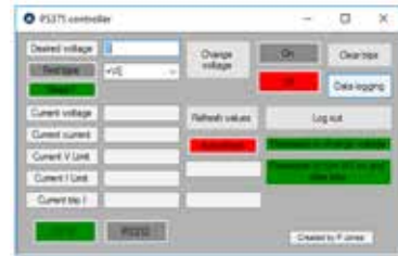
Figure 1: Graphical User Interface of the High Voltage Power Supply Controller
