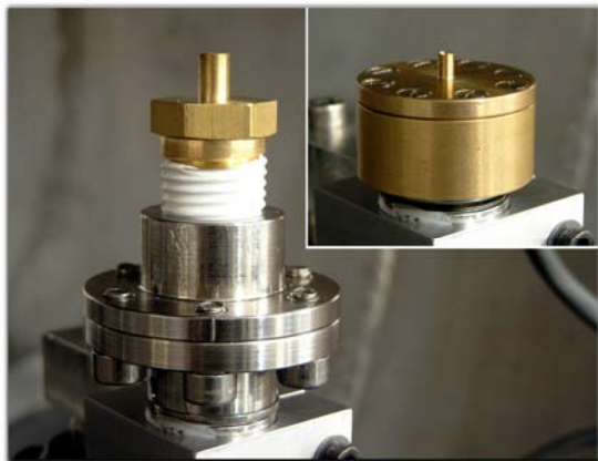
Figure 3. Image of Mach 3.5 nozzle head connected to series 9 valve. The inset shows the modified head applied with a Mach 5.5 nozzle. The outer diameters of the nozzles are 4.05 mm and 2.1 mm, respectively.
