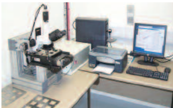
Figure 11. The Automated Scanning and Particle Counting Microscope system used to scan CR-39.
