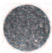
Figure 2. 2PPE image of Ge dots on Si(111) taken using the SH of the laser as the photon source. The field of view is 20 \mu m.
