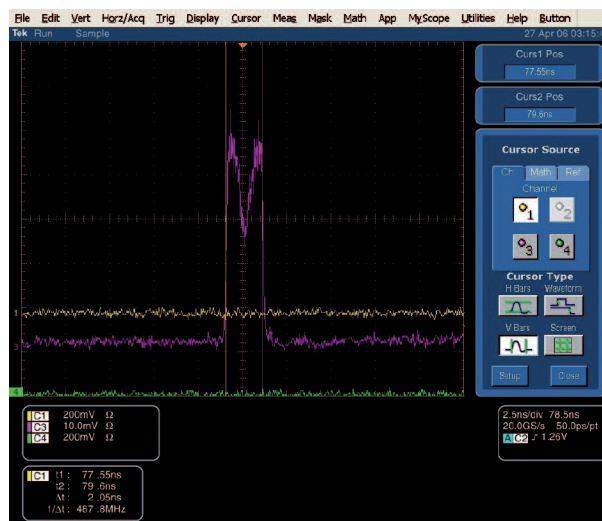
Figure 2. Shaped pulse from modulator – the data file has been modified to produce the 'M'.
