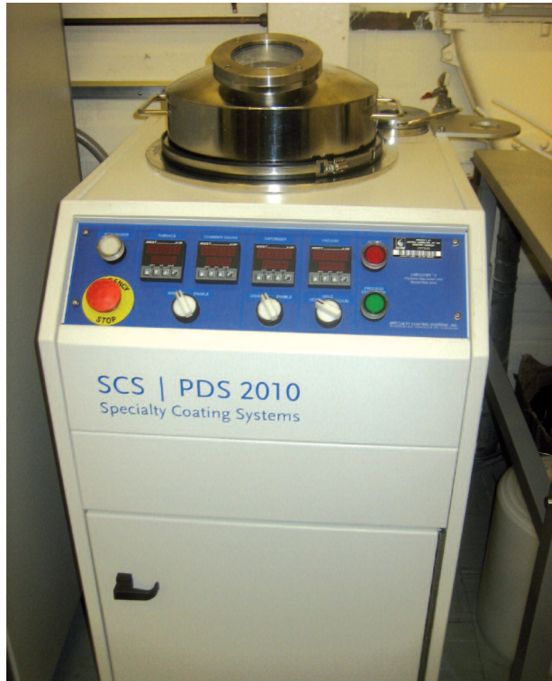
Figure 5. The parylene coater.
