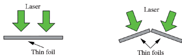
Figure 1. Schematic of the target design and laser beam geometry. Experiments compared the plasma outflow from the rear face of a planar target (left) to two angled planar targets (right).
