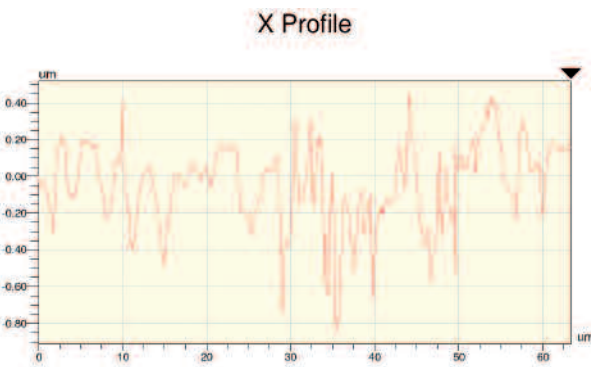
Figure 3. 2D lineout from the Wyko image of the glass surface at a magnification of 100 times over an evaluation length of 65 μm.
