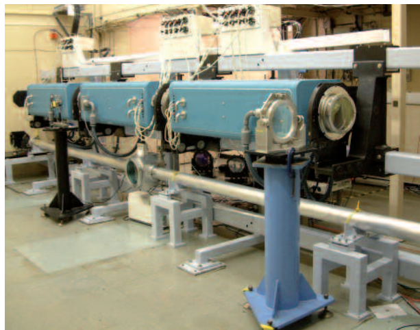
Figure 1. The beamline in LA4, the VSF for the long pulse beamline can be seen below the 208 mm diameter disc amplifiers.
