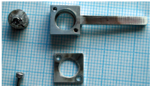
Figure 5. Post shot photograph of 4 mm thick Tungsten target and its holder. Background grid is defined by 1 mm squares.
