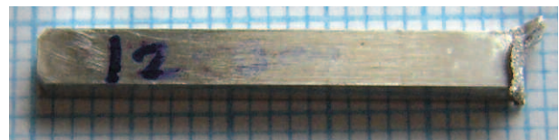
Figure 13. Aluminium stalk for mounting a 20 µm thick gold target after irradiation by part of the focussed beam. The material from the top millimetre of the stalk was vaporised and contributed to the debris plume shown in figure 10. Background grid is defined by 1 mm squares.
