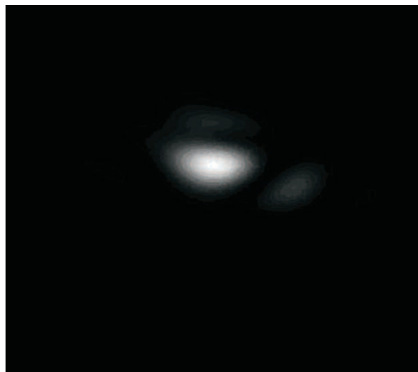
Figure 7. Full power focal spot imaged using the collection optics.
