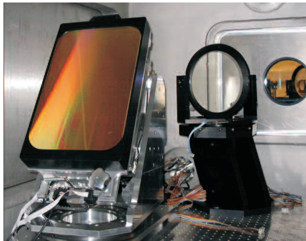
Figure 6. The second grating and its mount inside the compressor chamber.
