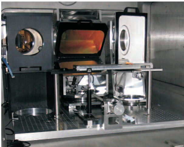
Figure 5. The first grating of the Gemini compressor mounted in the chamber, with the back mirror on the right.
