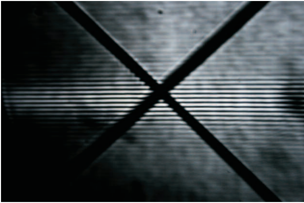
Figure 2. White light fringe pattern.
